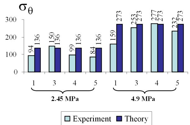
So, the acoustoelastic method, realized with the help of the device IN-5101A, has sustained check by an arbitrary calculative method with good results. This fact allows hope for successful introduction of this rather new perspective method in practice of the nondestructive evaluation of mechanical stresses in engineering materials.
