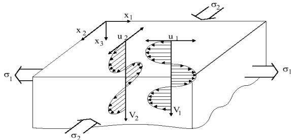
Combined equations (1,2) provide the evaluation of stresses in accordance with the nonlinear elastic properties of testing material and the results of precise time-of-flight measurements of shear and longitudinal ultrasonic waves:
